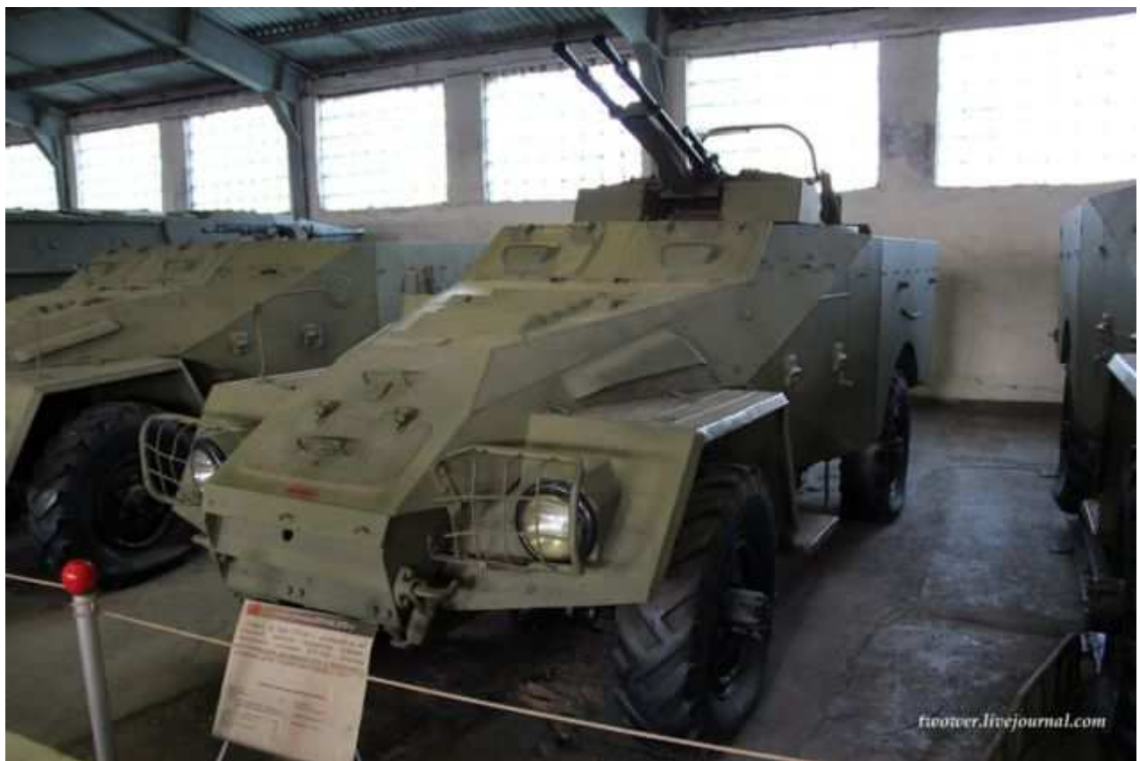
BTR-40A – Kubinka Tank Museum (Russia) SPAAG version armed with twin ZPTU-2 14.5mm twin anti-aircraft gun
