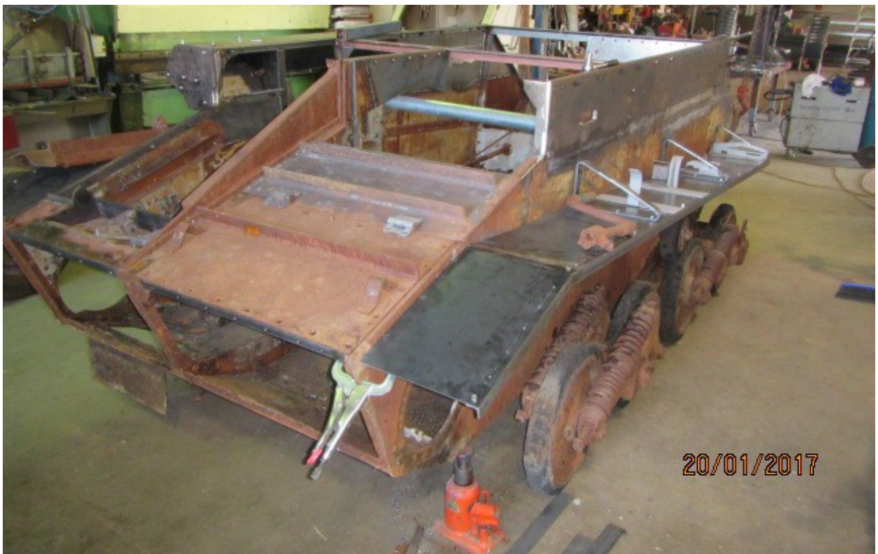
Vickers-Carden-Loyd Light Tank Mk VI hull – Colin Jones Collection, Adelaide (Australia) Ex-John Belfield collection
