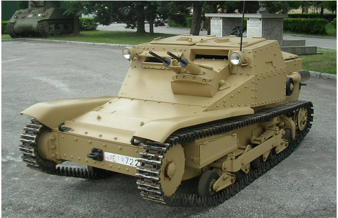
L3/35 – Caserma "De Carli", Cordenòns (Italy) – running condition Restored with a modern engine from a FIAT Campagnola AR 70 and incorrect engine's cowling
