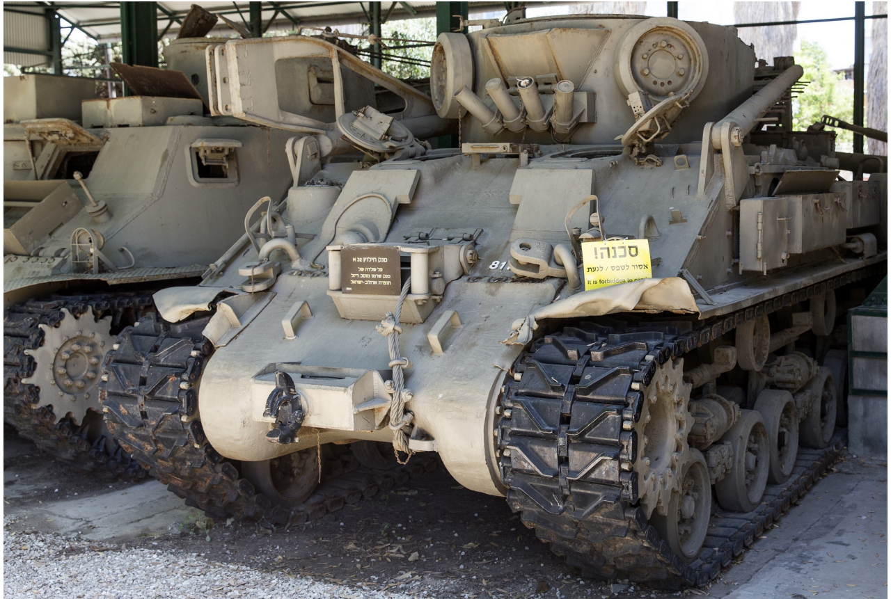
M32A1B3 TRV – Batey ha-Osef Museum, Tel Aviv (Israel) Converted from a Ford M4A3. This tank has got the automatic tow hook modification in 1945
