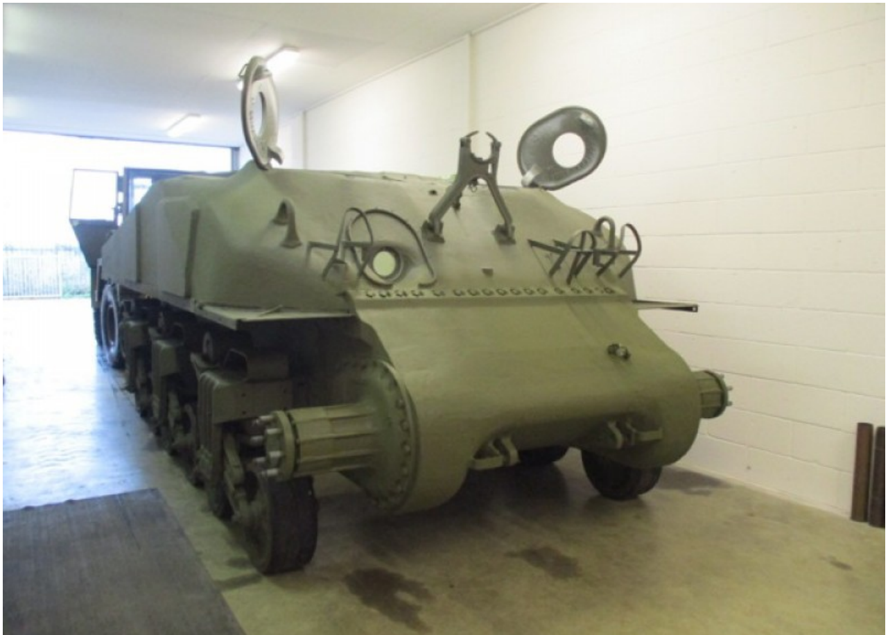
Large Hatch M4(75) Composite Sherman – Private collection (UK) Serial Number 5964x, built by Chrysler in January, 1944. This tank seems to come from Brazil
