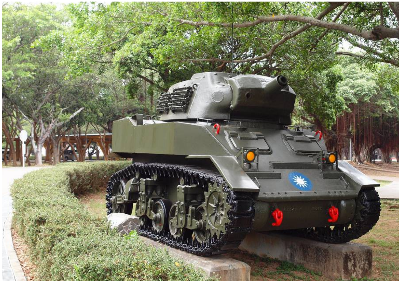
M8 Howitzer Motor Carriage – Ch'eng-kung-ling, Nantun District, Taichung (Taiwan) The mantlet comes from an M24 Chaffee
