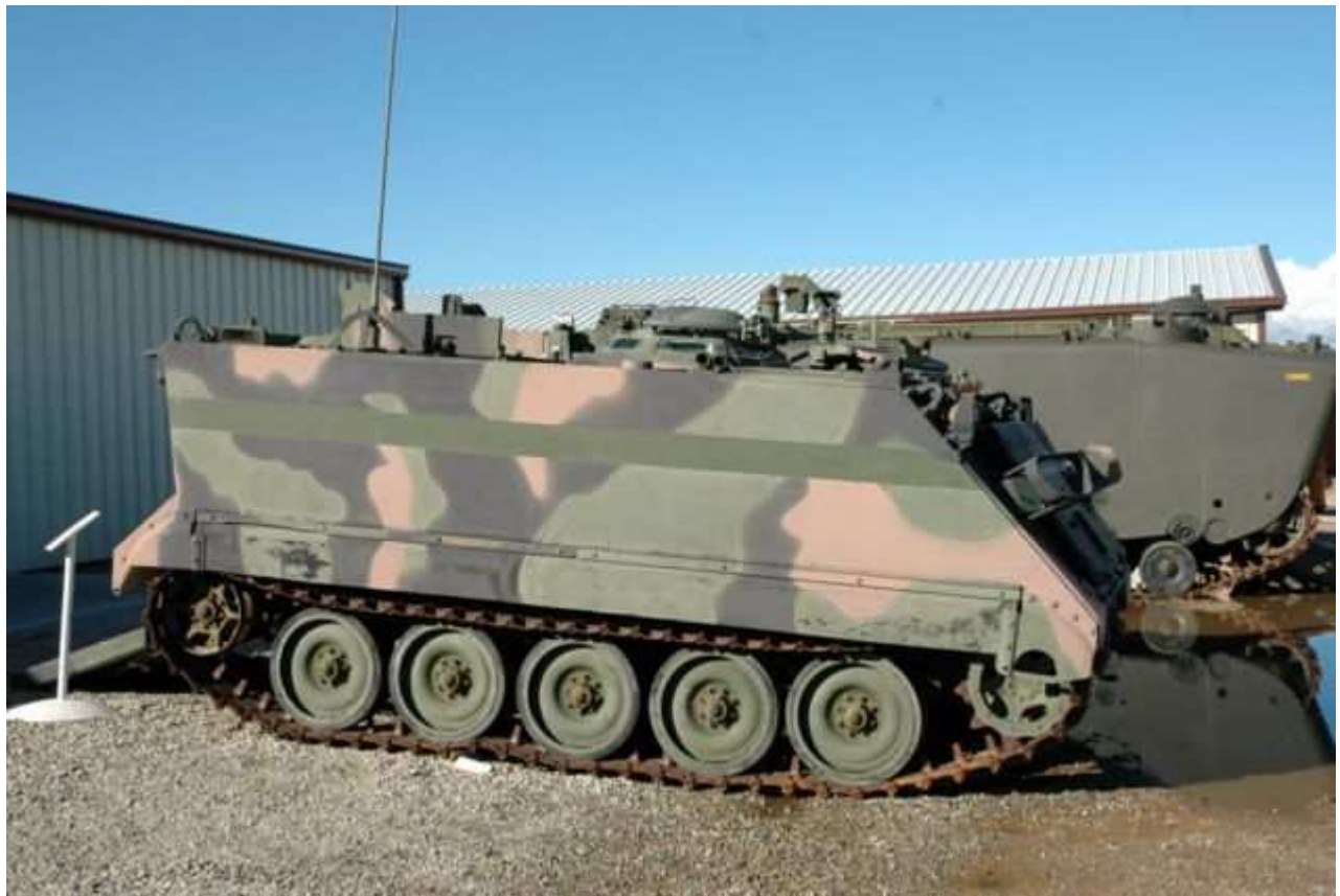
M901 – Estrella Warbirds Museum, Paso Robles, CA (USA) TOW launcher turret is missing
