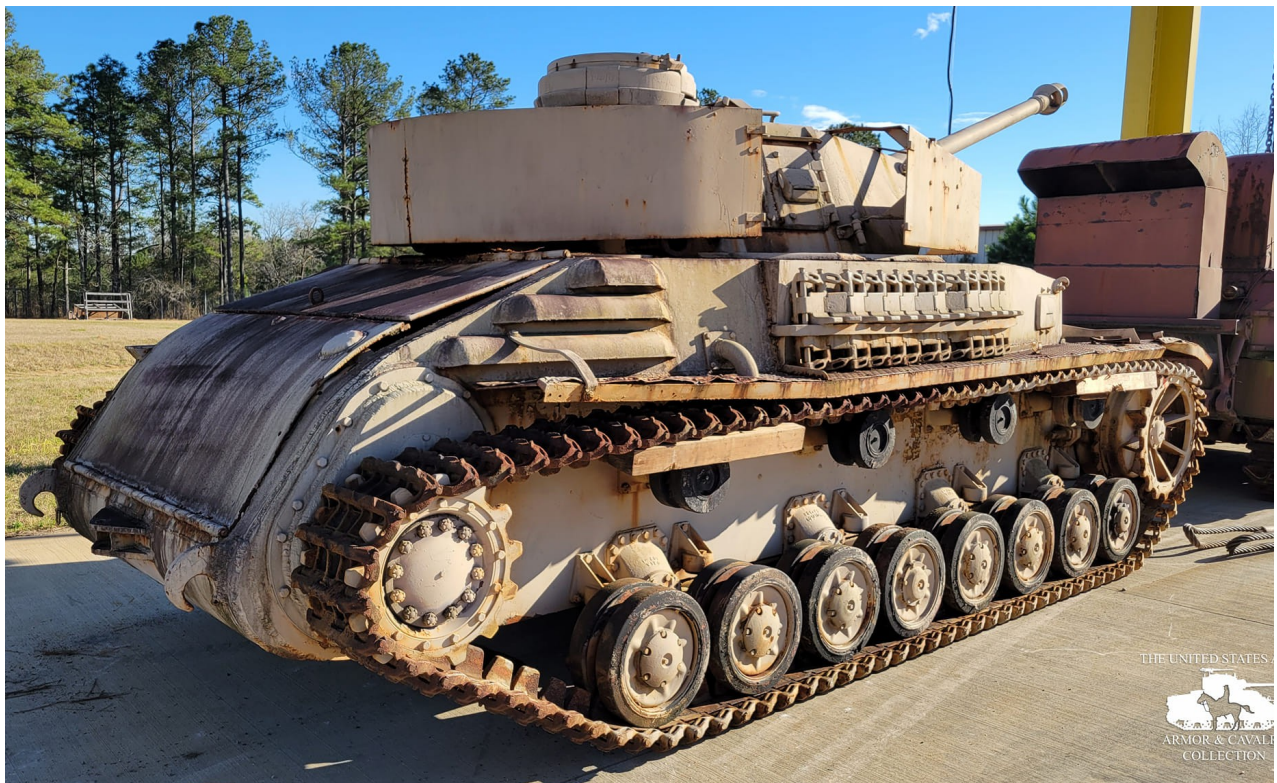
PzKpfw. IV Ausf. G with Thoma experimental hydraulic drive U.S. Army Armor & Cavalry Collection, Fort Benning, GA (USA) Formerly part of the Aberdeen proving ground museum
