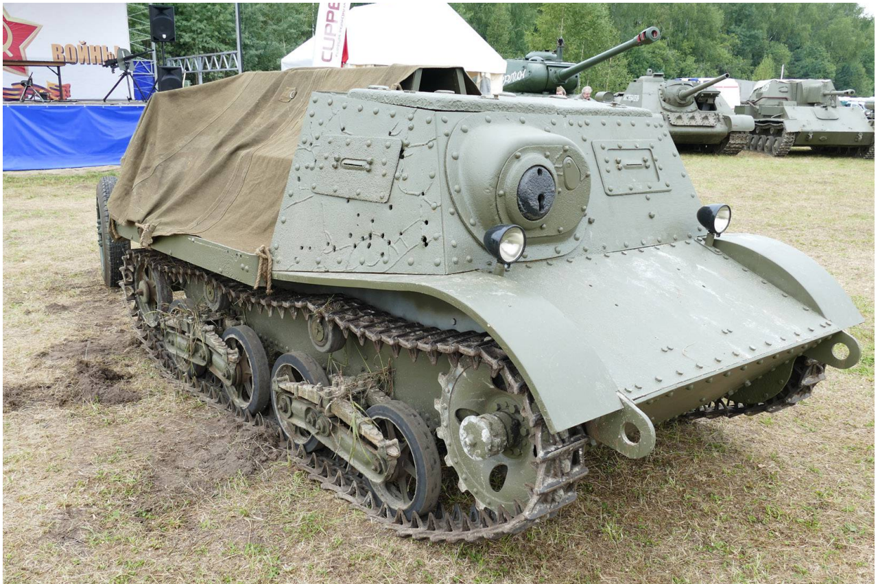
T-20 Komsomolets – Caponier Club Collection, Moscow (Russia) – running condition Rebuilt from the remains of tanks completely destroyed during the war, which were found by search teams on the battlefields
