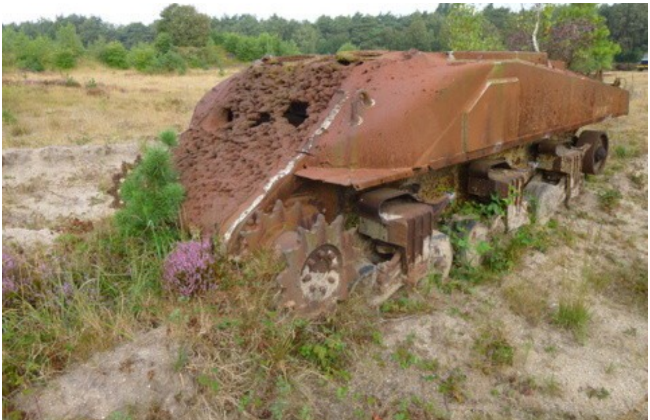
Second Sherman Hybrid Ic hull – Groot Schietveld Range, Brasschaat (Belgium) SN 44533, built by Chrysler in October, 1943. Hull heavily damaged by anti-tank weapons (Michel van Loon)
