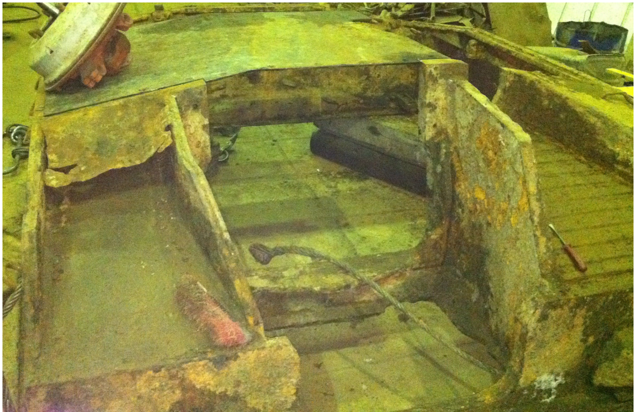
Sturmgeschütz III Ausf. B upper hull – Dmitry Bushmakov Collection (Czech Republic) This Stug upper hull came from Zavidovo region (Tver Oblast)
