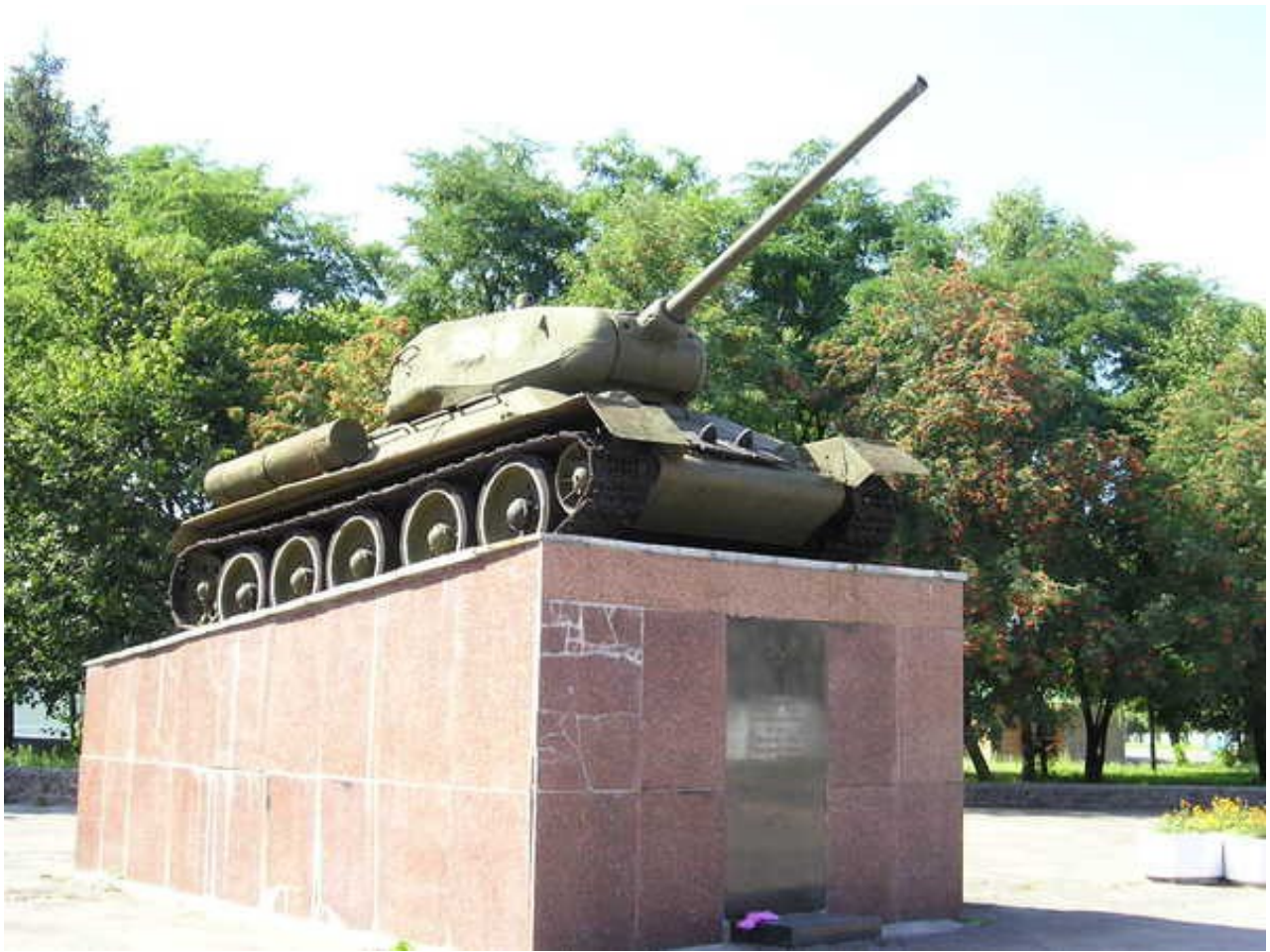
T-44 turret on T-34 hull – Ovruch, Zhytomyr Oblast (Ukraine)
