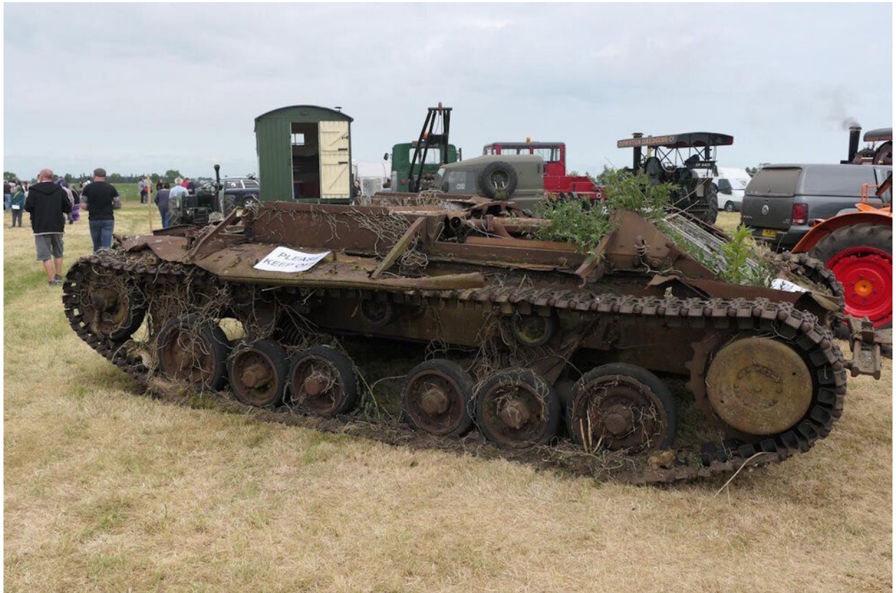
Valentine IX Duplex Drive lower hull – Private Collection (UK)
